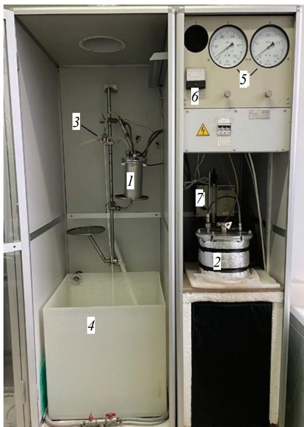
**Fig. 1.** Setup for the hollow fiber membrane fabrication: (1) spinning dope vessel; (2) internal coagulant bath; (3) spinneret; (4) receiving bath; (5) pressure gauges; (6) bore fluid temperature sensor and (7) thermostat
