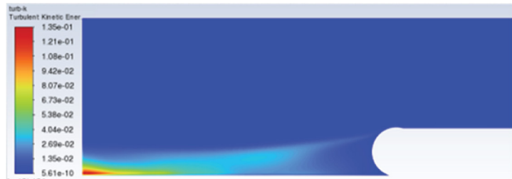
Fig. 11. Turbulence distribution at e_2/D = 0.98 , Re = 3.2 \cdot 10^5
