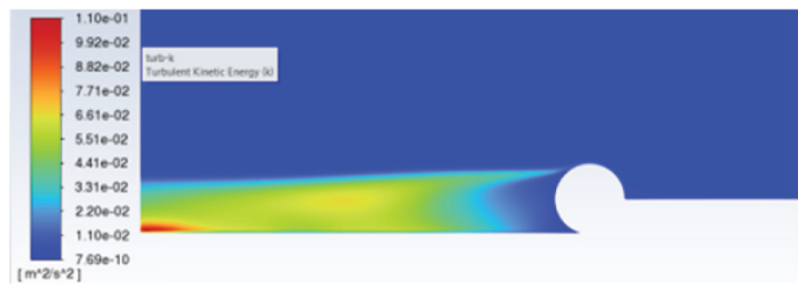
Fig. 9. Turbulence distribution at e_2/D = 0.5 ; Re = 3.2 \cdot 10^5
