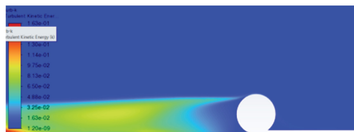
Fig. 7. Turbulence distribution at e_2/D = 0.1 ; Re = 3.2 \cdot 10^5
