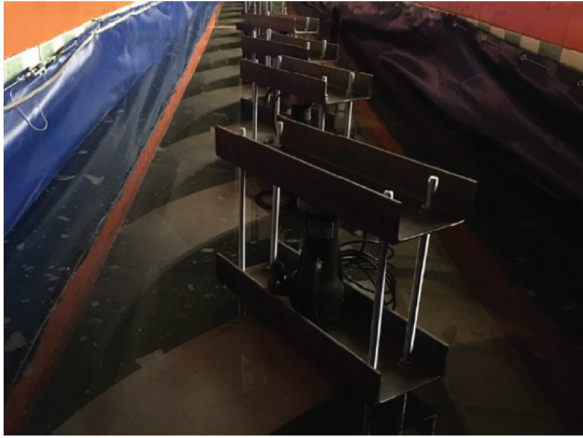
Fig. 2. Pipe samples installed in the space of a tray filled with water
