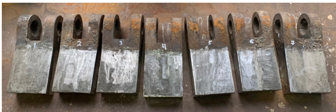
Fig. 3. Visual inspection of the beater surface after removal of metallurgical slag
