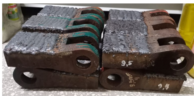
Fig. 11. Surfaced beaters for mill mounting
