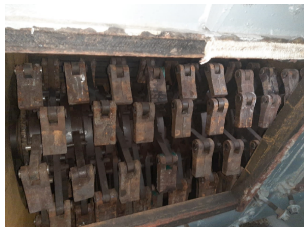
Fig. 12. Placement of beaters in the mill
