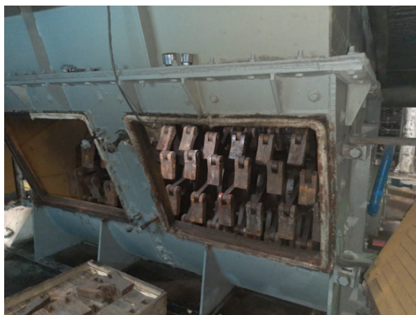
Fig. 12. Placement of beaters in the mill
