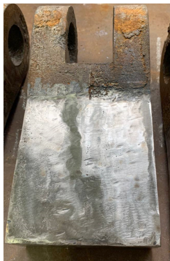
Fig. 1. Original beater component for surfacing
