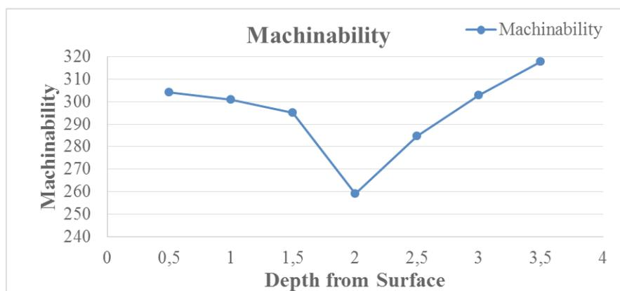
Fig. 3. Machinability at different depth from M-M interface
