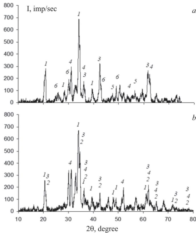
Fig. 2. Diffractograms of slags in the production of bismuth lead:
