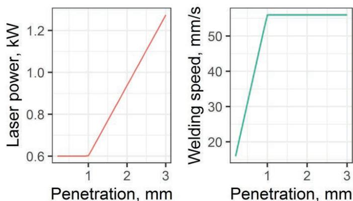
Fig. 5. Optimal laser power and welding speed depending on the weld penetration
