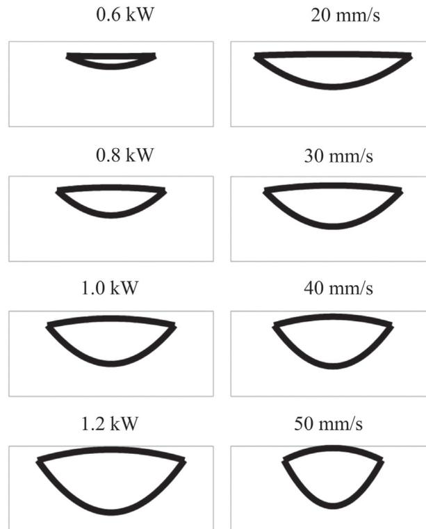
Fig. 3. Calculated shape of the weld seam depending on laser power and welding speed:
