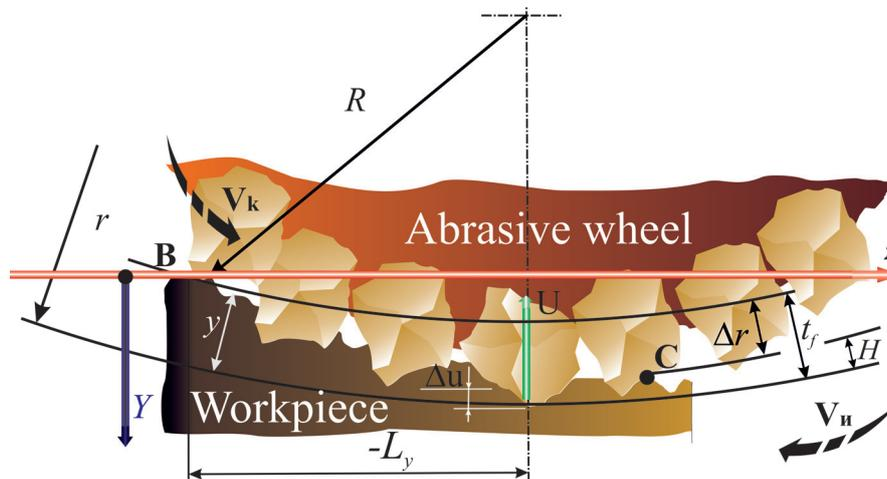
Fig. 2. Scheme for calculating the number of tops of abrasive grains, passing through a unit surface area by the thickness of the tool per unit of time
