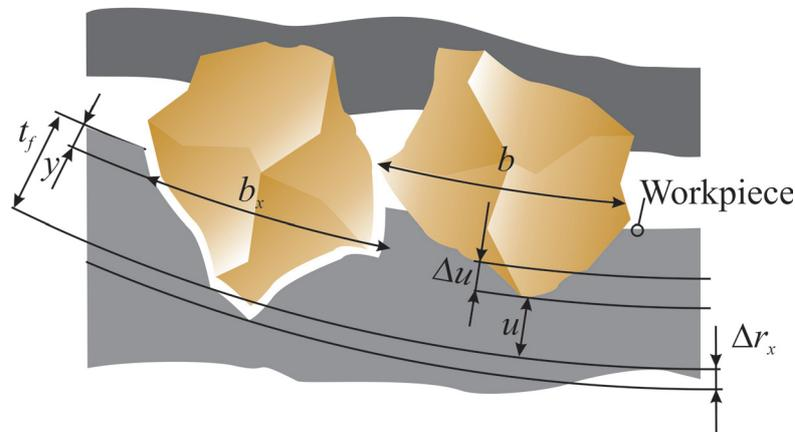
Fig. 4. Scheme of interaction of abrasive grains with a ceramic workpiece
