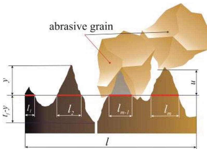
Fig. 1. Scheme for calculating the probability of removing the surface layer when grinding the material
