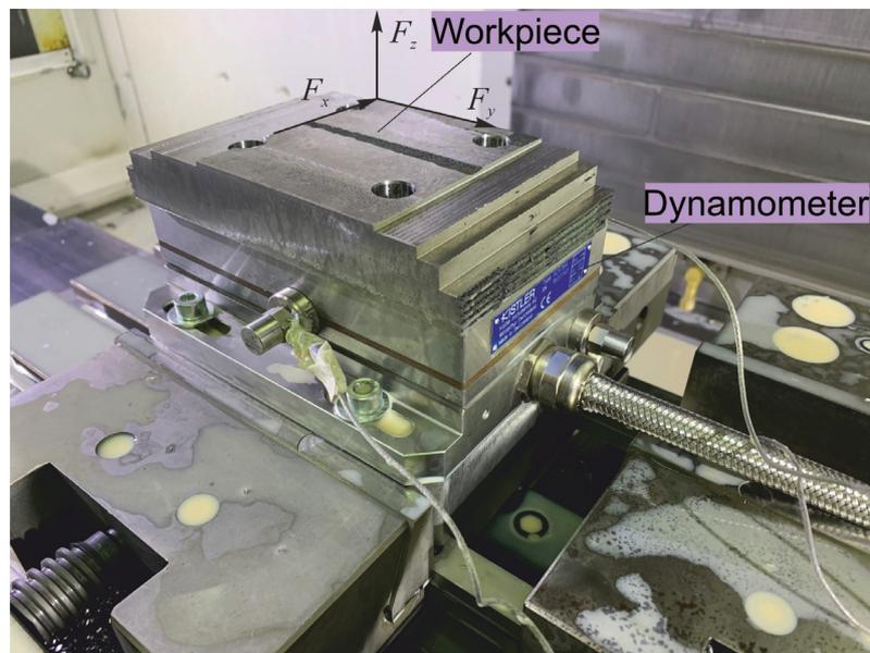
Fig. 1. Workpiece clamped in the dynamometer
