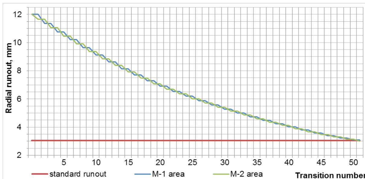
Fig. 11. Graph of the change in the  $\Delta_{ECR}^k$  value of the cross sections of the processed surface areas *M-1* and *M-2* from the 1<sup>st</sup> to the 51<sup>st</sup> transition inclusive
