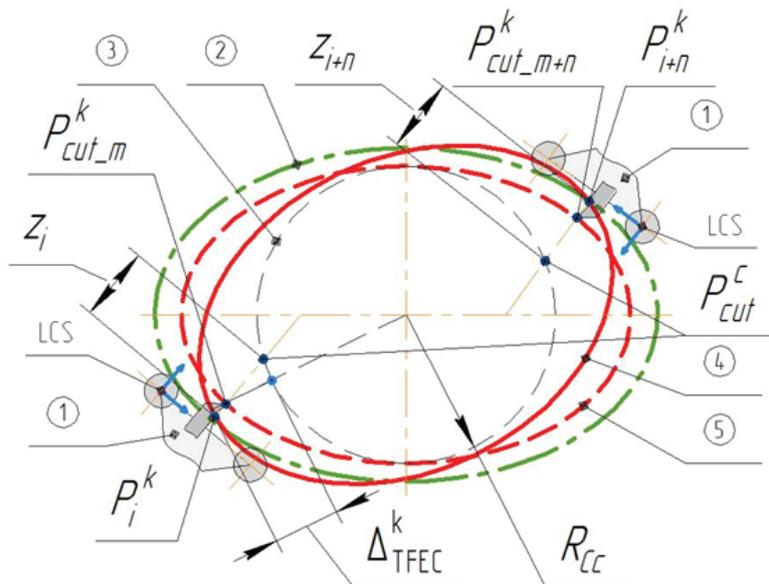
Fig. 4. Schematic diagram of calculating the depth of cut in the  $k^{th}$  section
