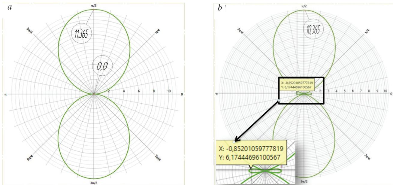
Fig. 10. Round diagram of the shape deviation of the cross-sectional contour of the machined area after the 2<sup>nd</sup> transition:
