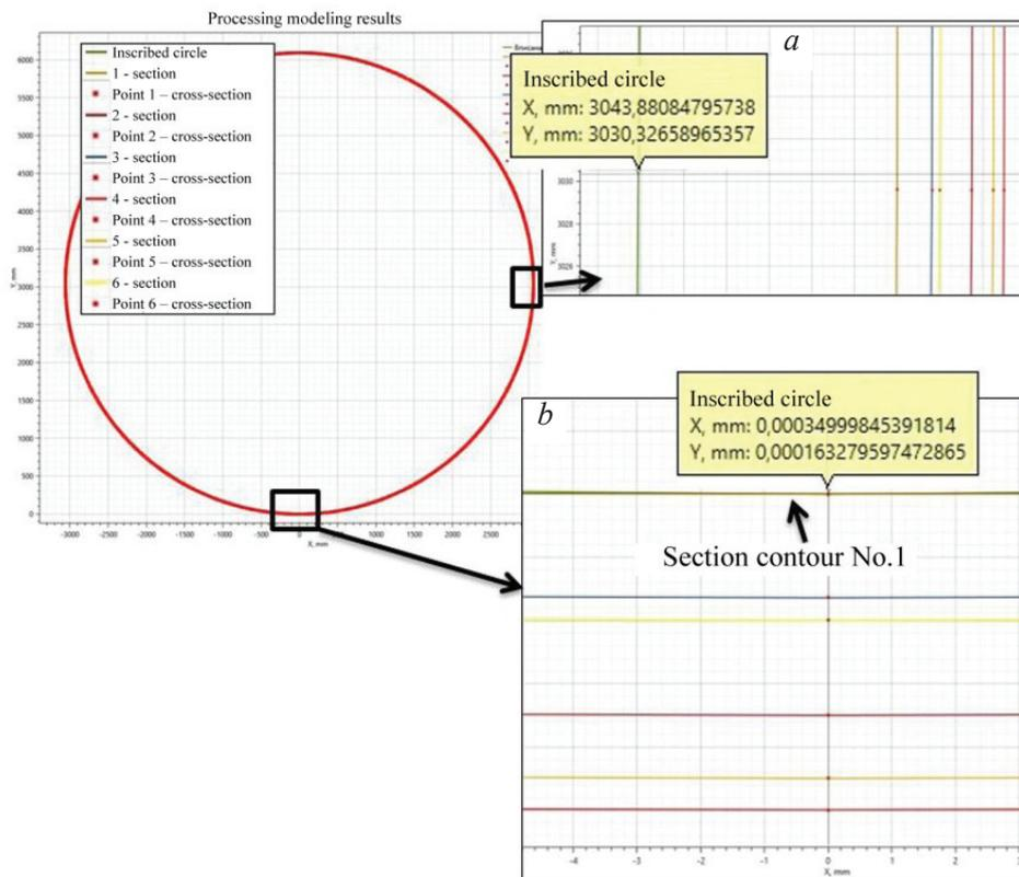
Fig. 7. Combined diagram of the contours of the sections and the inscribed cylinder:
