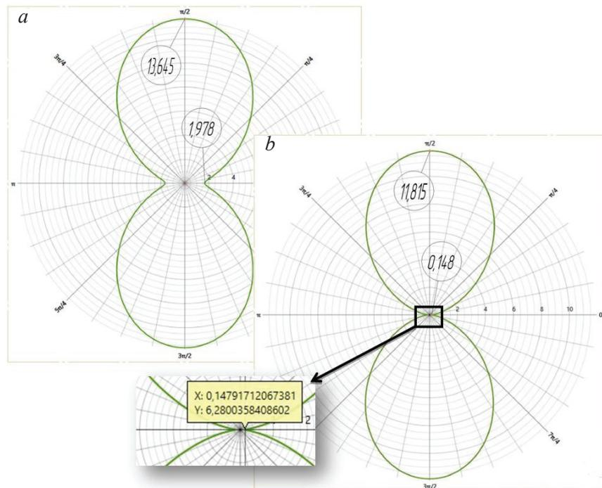
Fig. 9. Round diagram of the shape deviation of the contour of the processed surface area at the 1<sup>st</sup> transition:
