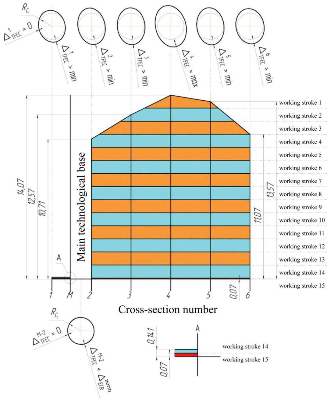
Fig. 12. Distribution of maximum allowances for processing a surface area on a working stroke of the 52<sup>nd</sup> transition
