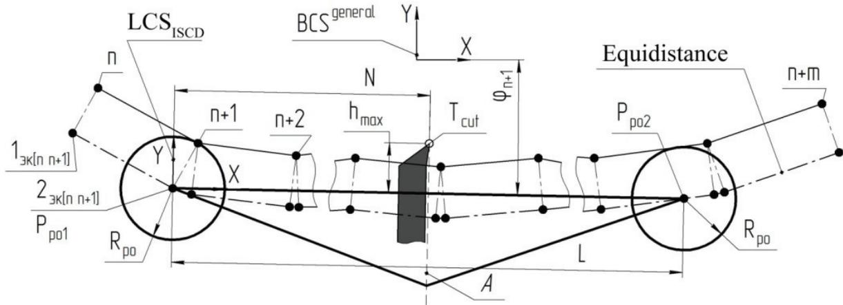
Fig. 2. Schematic diagram of the calculation of the processing module position (A – line corresponding to the axis of movement of the cutting tool edge)
