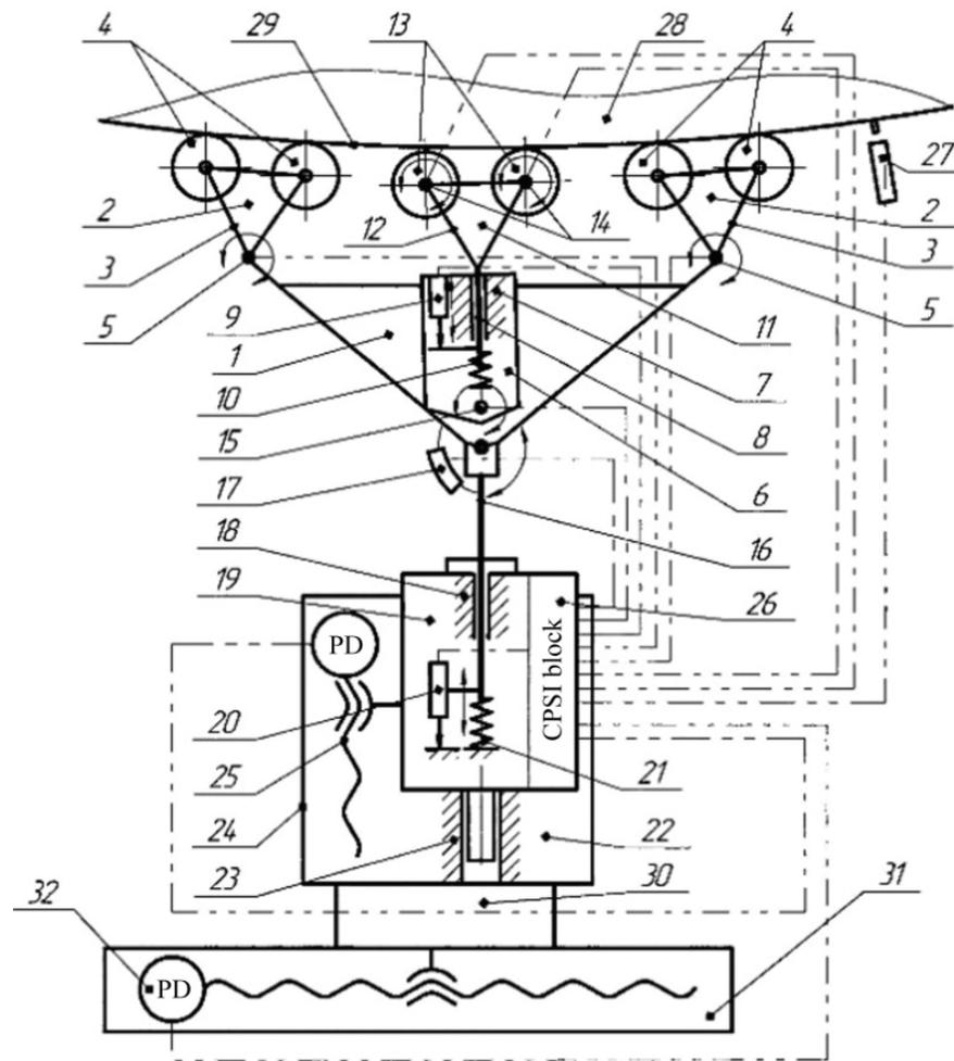
Fig. 13. Device for measuring product shape parameters:
