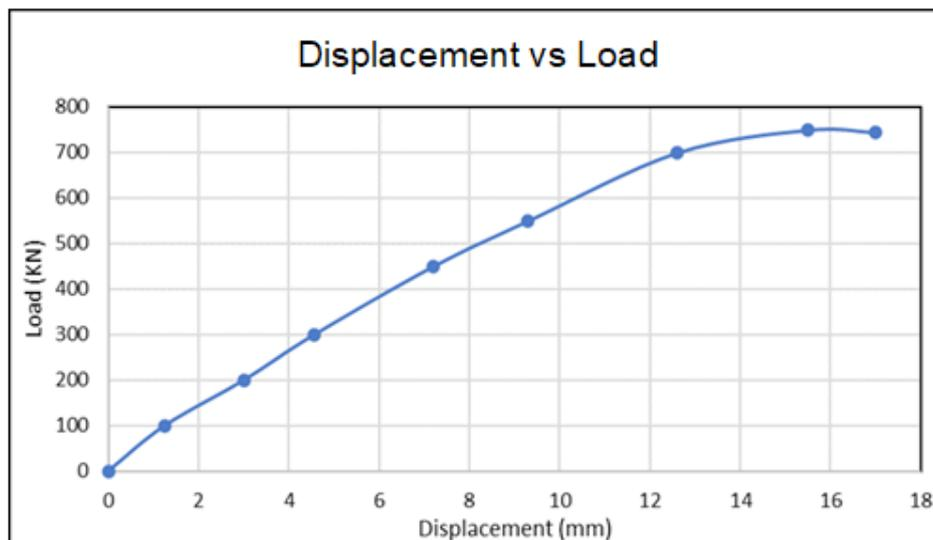
Fig. 11. Graph for dependency of displacement (mm) on load (kN) of the foam aluminium material specimen
