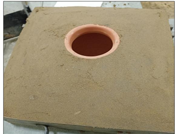
Fig. 3. Clay pot mould
