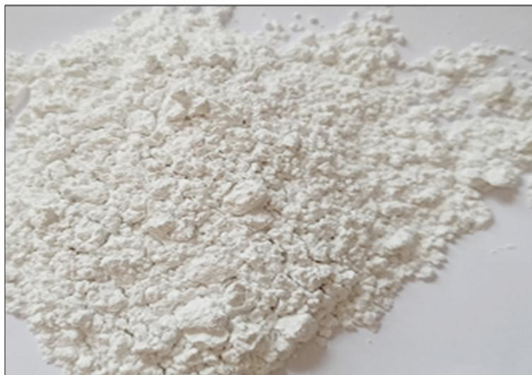
Fig. 1. General view of calcium carbonate particles used as a foaming agent
