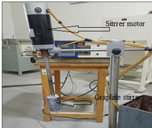
Fig. 2. Stir casting setup
