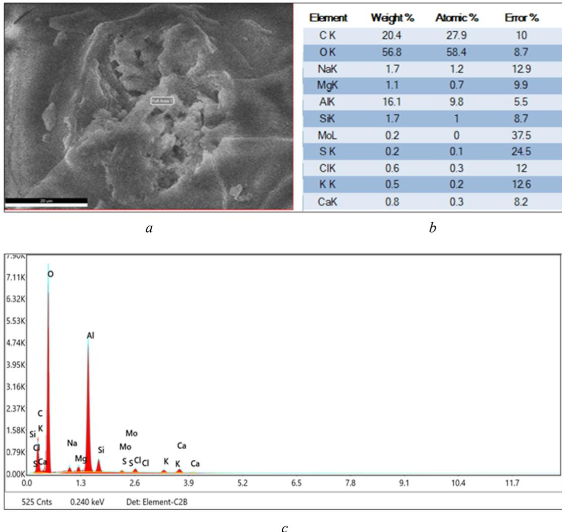
Fig. 9. Elemental analysis of aluminium foam (*a*) mapping area, (*b*) weight %, (*c*) elemental spectra
