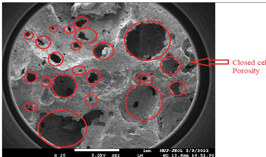
Fig. 7. Surface morphology of closed-cell aluminium foam (2.5 % calcium carbonate), observed using *FE-SEM*, is characterized by interconnected pores
