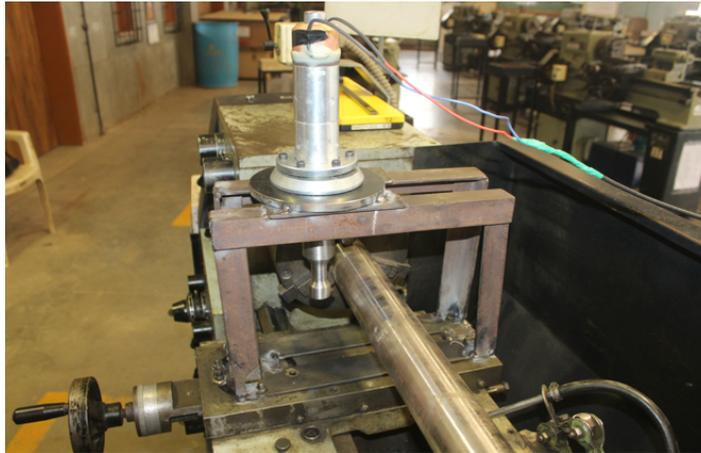
Fig. 4. Actual photograph of base frame with *UVAHT* mounting
