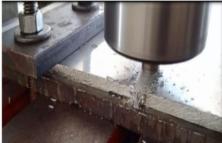
Fig. 2. Material flow during FSW
