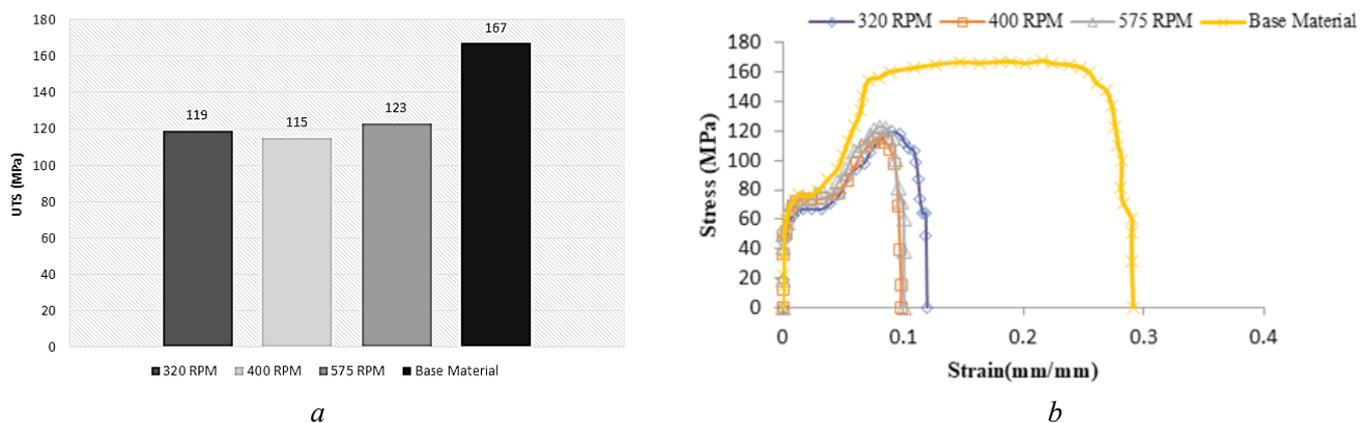
Fig. 8. Tensile test results of welds fabricated by cylindrical taper pin profile:
