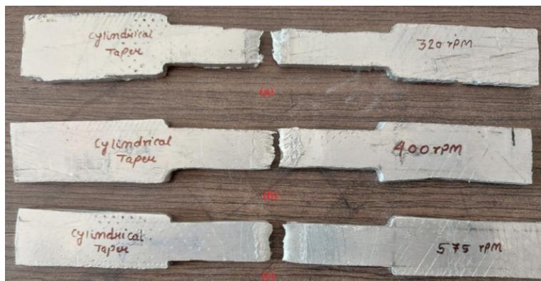
Fig. 7. Fractured specimens after tensile test of joints fabricated using taper cylindrical pin
