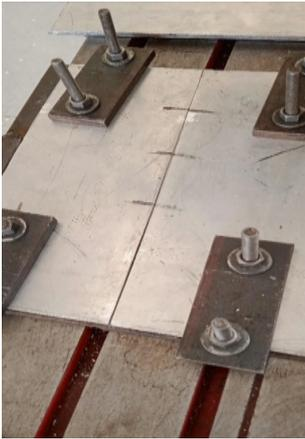
Fig. 1. Plates mounted on the bed of vertical milling machine
