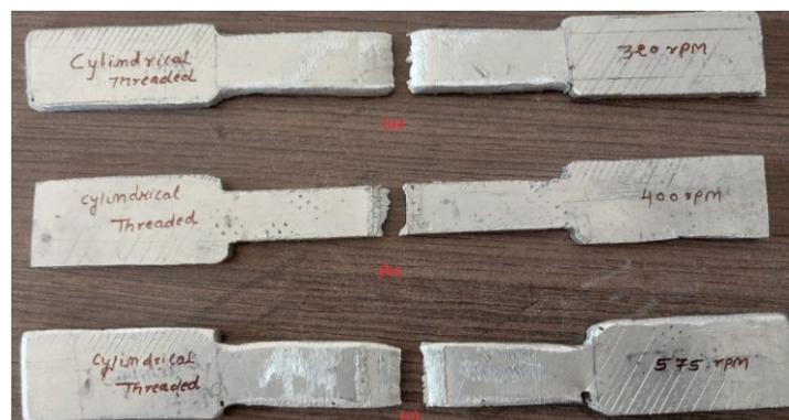
Fig. 5. Fractured specimens after tensile test of joints fabricated using threaded cylindrical pin
