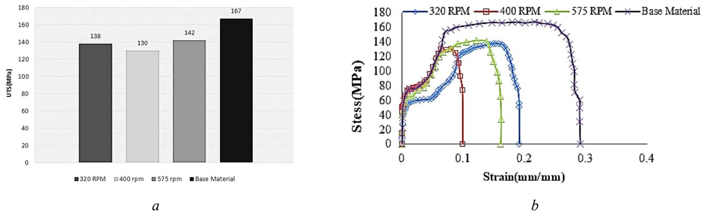
Fig. 6. Tensile test result of weld fabricated by cylindrical threaded pin profile:
