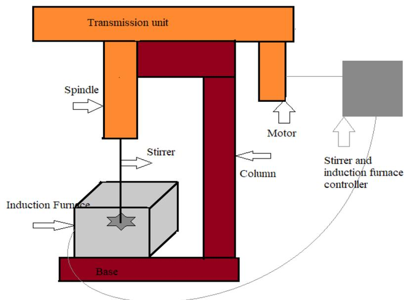
Fig. 3. Stirrer casting setup [12]
