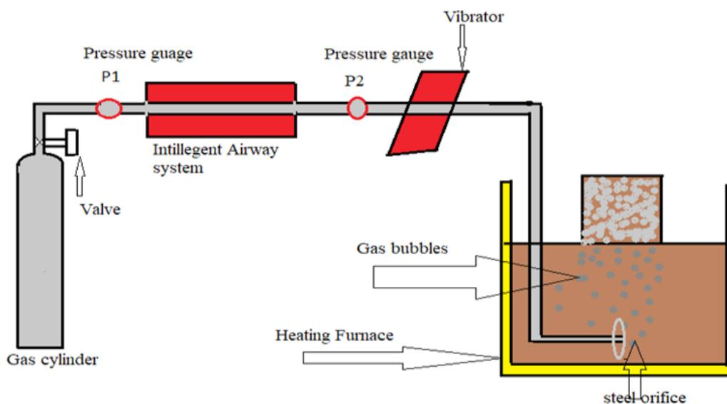
Fig. 2. Melt gas injection method [8]
