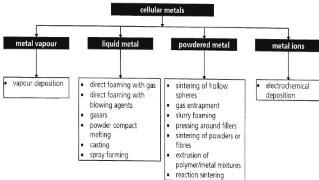
Fig. 1. Metal foam production methods [3]
