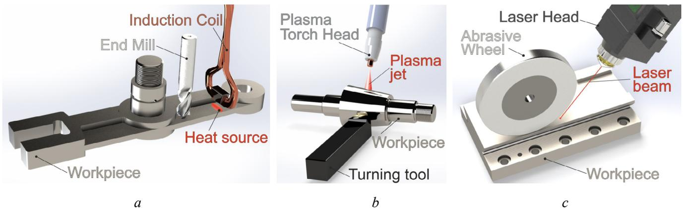
Fig. 1. Varieties of hybrid metalworking machines that combine machining with various heat sources: a – Induction Assisted Milling (IAM); b – Plasma Assisted Turning (PAT); c – Laser Assisted Grinding (LAG)
