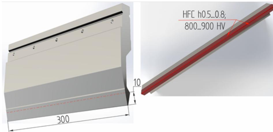
Fig. 3. Press brake plug
