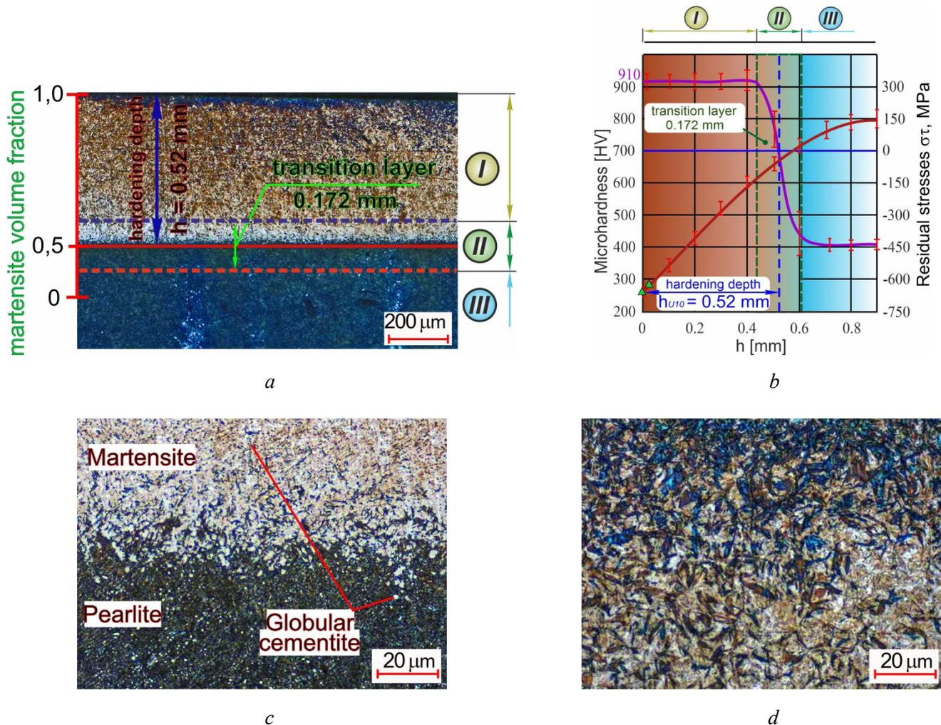
Fig. 10. Experimental results for parts made of U10A steel:
