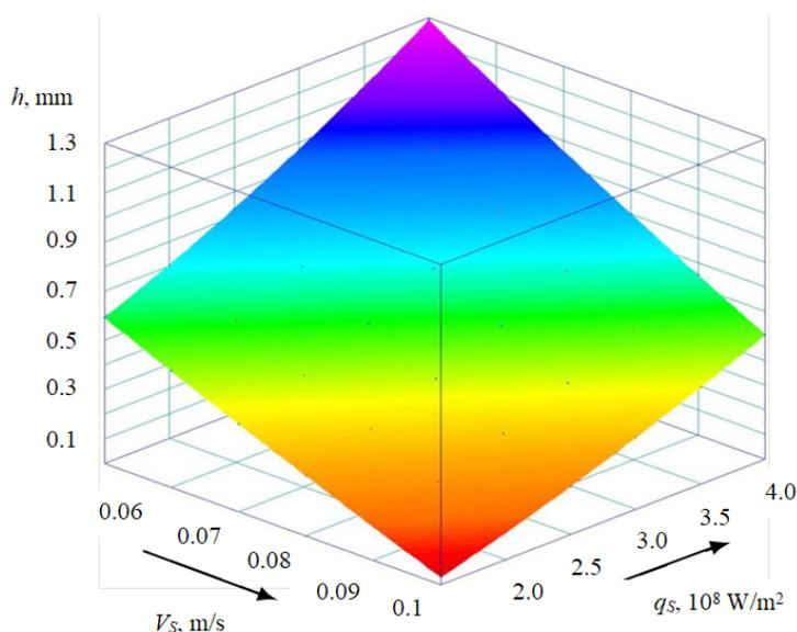
Fig. 7. Functional dependence  $h(q_s, V_s)$  for *U10A* steel
