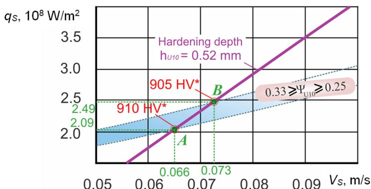
Fig. 9. The dependence of specific power of the source on its speed while HEH HFC hardening steel U10 to a depth of  $h = 0.52$  mm.
