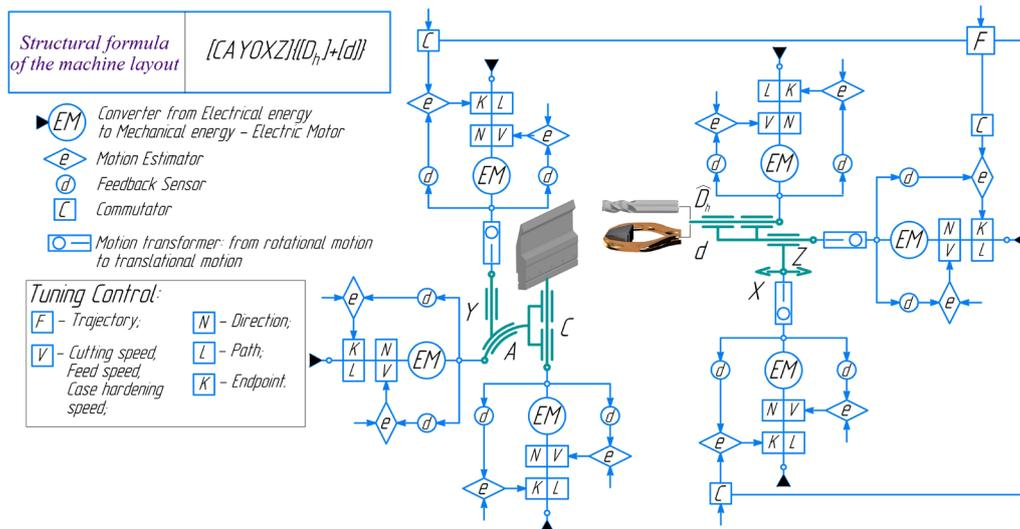
Fig. 4. Block schematic diagram of the hybrid metalworking machine
