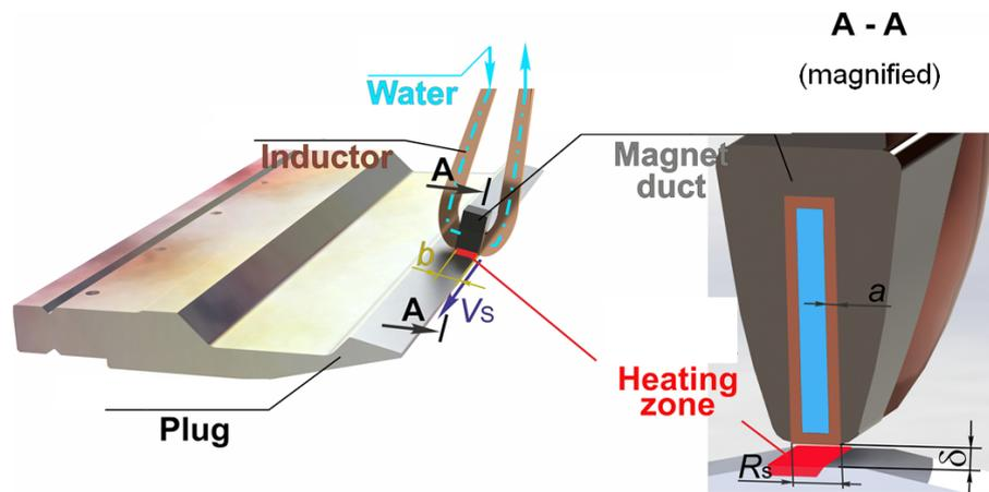
Fig. 2. Pattern of HEH HFC hardening of a punch
