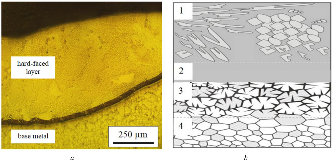
Fig. 2. Micrograph (a) and scheme (b) of the 1<sup>st</sup> specimen cross section structure after plasma-jet hard-facing: 1 – hypereutectic zone with iron borides of various structures; 2 – eutectic zone; 3 – heat affected zone; 4 – base metal
