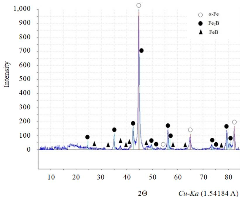
Fig. 3. X-ray pattern of the first specimen after plasma-jet hard-facing
