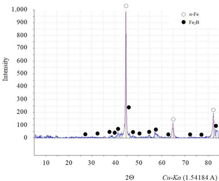
Fig. 8. X-ray pattern of the 3<sup>rd</sup> specimen after plasma-jet hard-facing
