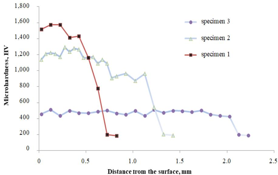
Fig. 10. Distribution of microhardness over the depth of hardened layers
