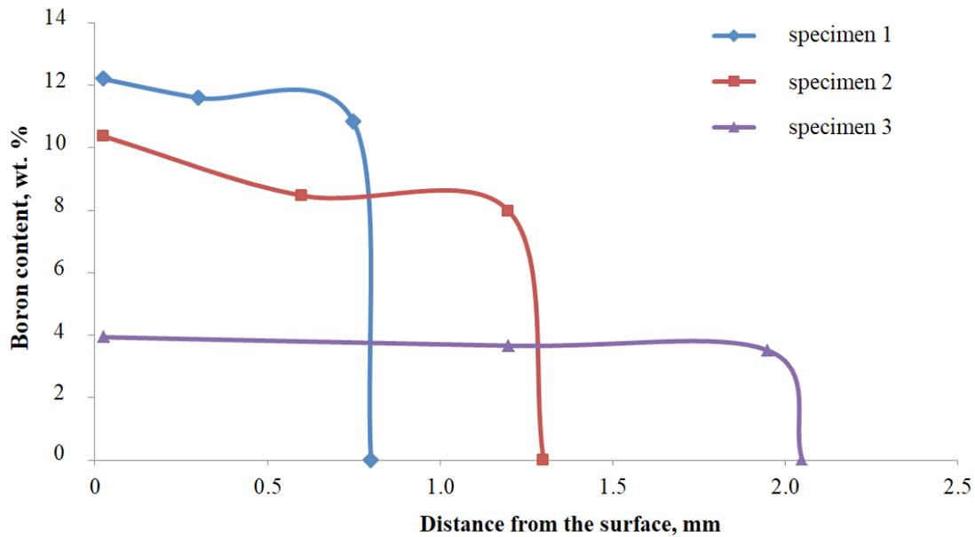
Fig. 9. Distribution of boron over the layer depth on steels after plasma-jet hard-facing
