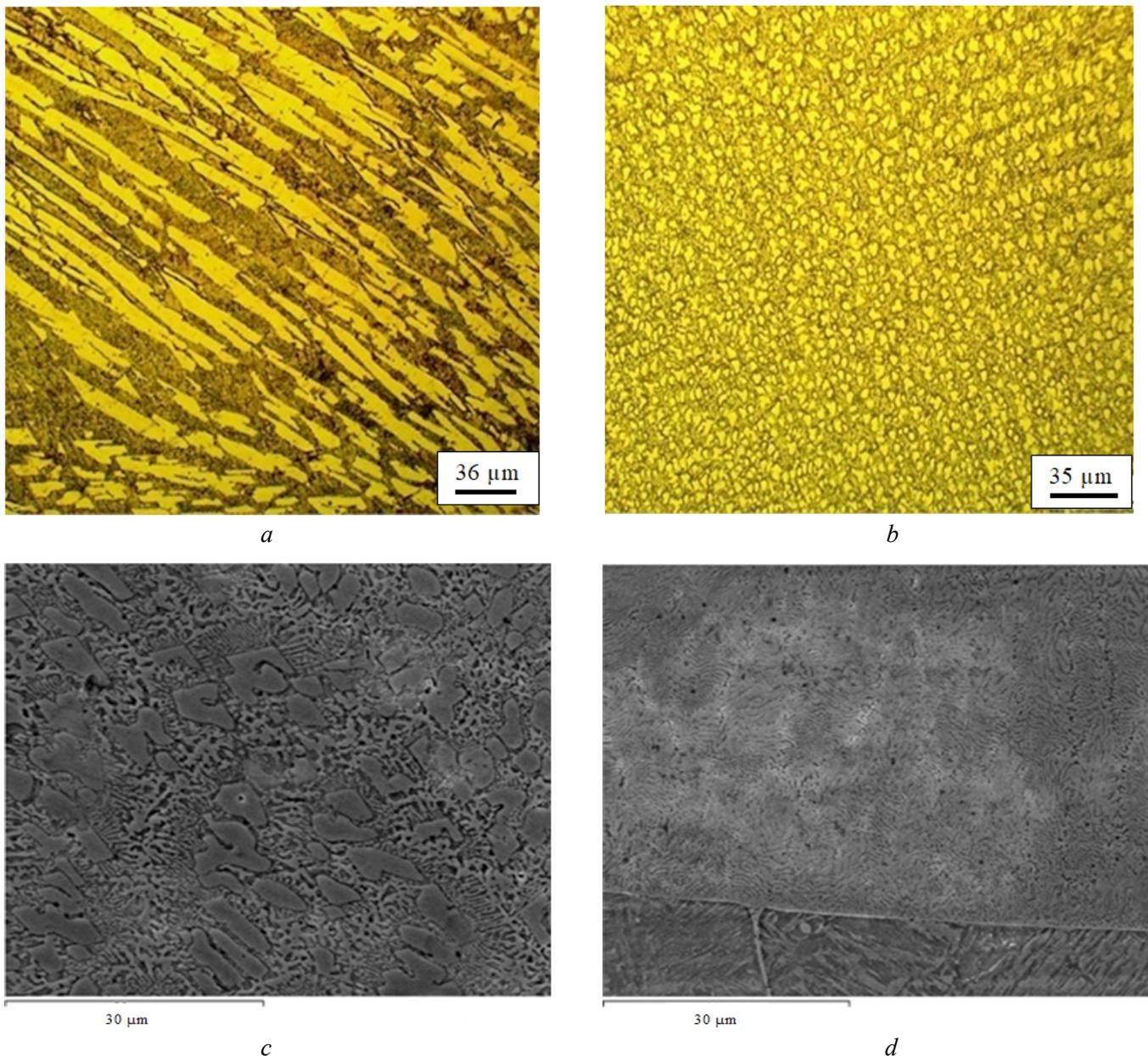
Fig. 5. Microstructure of the 2<sup>nd</sup> specimen after plasma-jet hard-facing:
