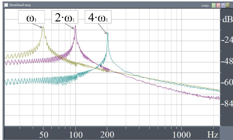
Fig. 6. Frequency response of harmonic sound waves obtained by milling with an inclination angle of  $40^\circ$  (Formulated by the authors)
