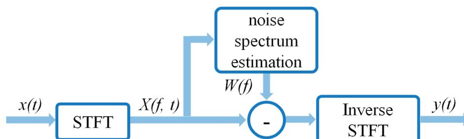
Fig. 2. The proposed spectral subtraction algorithm scheme:
