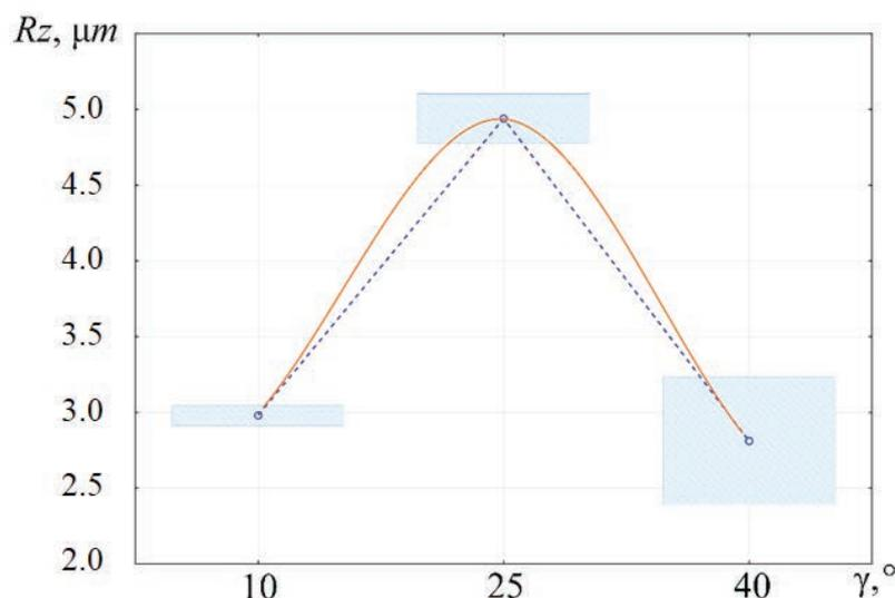
Fig. 8. Parameter  $Rz$  depending on the machining angle for a double-tooth cutter (Formulated by the author)
