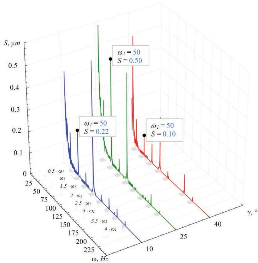
Fig. 4. Comparison of the frequency spectrum after milling with different angles of inclination,  $z = 2$  (Formulated by the authors)
