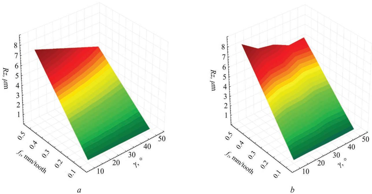
Fig. 9. Dependences of the roughness  $R_z$  on the feed and the angle of inclination of the tool:
