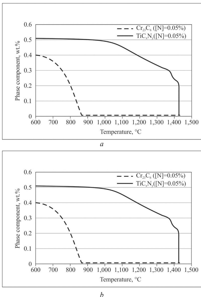
Fig. 1. Dependence of the content of chromium carbides  $Cr_{23}C_6$  and titanium carbonitrides  $TiC_xN_y$  on the nitrogen content in steel:
