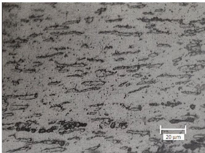
Fig. 3. Microstructure of a rod Ø 3 mm made of steel grade *12-Cr18-Ni10-Ti* after austenization
