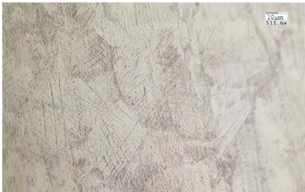
Fig. 2. Occurrence of martensitic  $\alpha$ -phase in steel *12-Cr18-Ni10-Ti*, rod Ø4 mm
