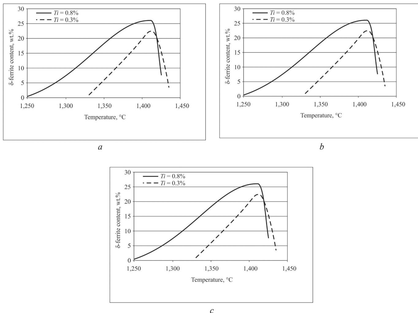
Fig. 4. Dependence of the content of  $\delta$ -ferrite in steel *12-Cr18-Ni10-Ti* at different alloying contents: a – the effect of titanium; b – the effect of chromium; c – the effect of carbon
