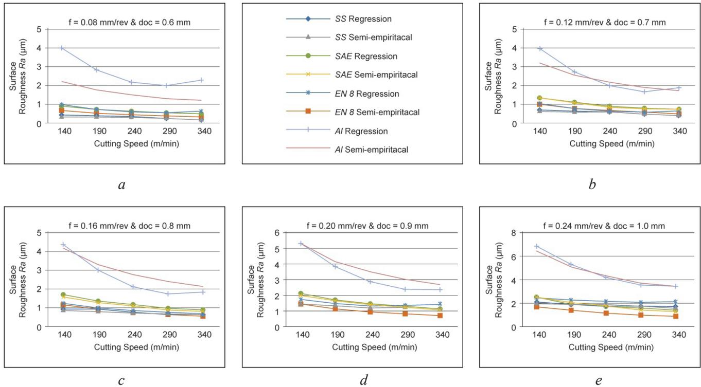
Fig. 4. Effect of cutting speed on surface roughness at different feed rate and depth of cut for all materials using *TiAlN*-coated tool
