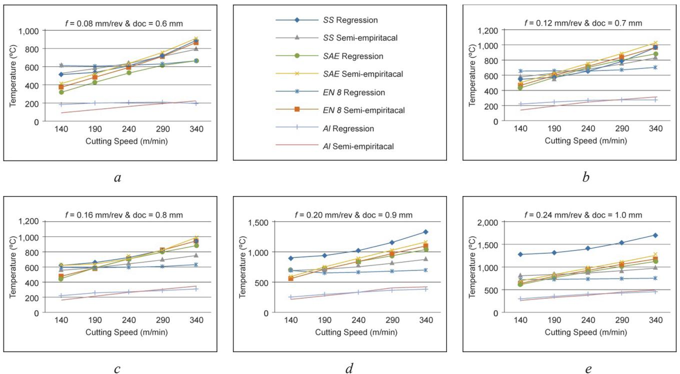
Fig. 8. Effect of cutting speed on cutting temperature at different feed rate and depth of cut for all material using  $TiAlN$ -coated tool
