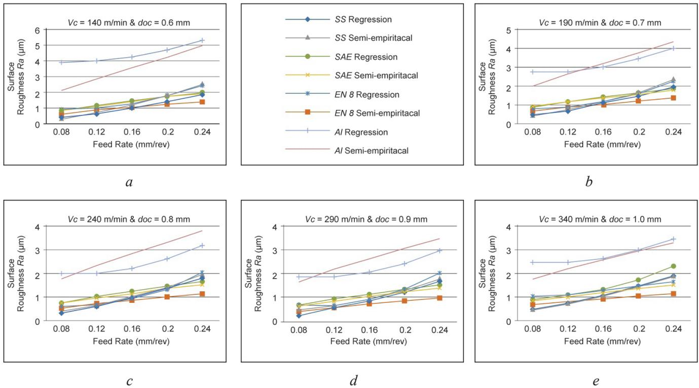
Fig. 3. Effect of feed rate on surface roughness at different cutting speed and depth of cut for all materials using  $TiAlN$ -coated tool
