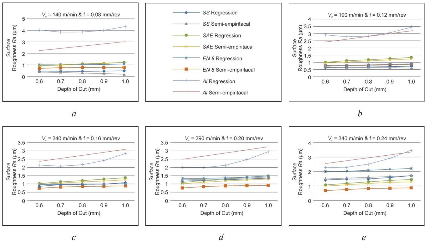
Fig. 5. Effect of depth of cut on surface roughness at different feed rate and cutting speed for all materials using *TiAlN*-coated tool
