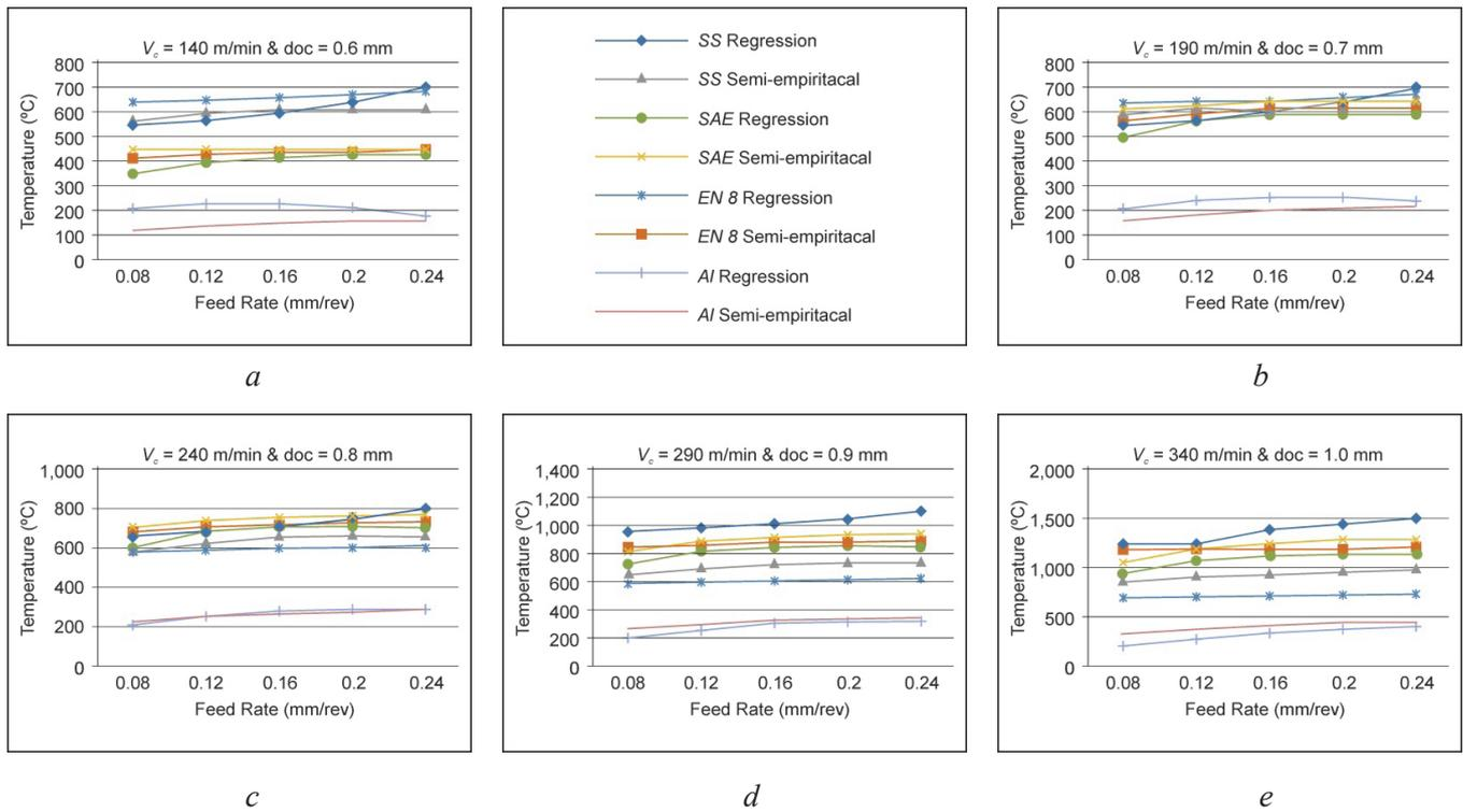
Fig. 7. Effect of feed rate on cutting temperature at different cutting speed and depth of cut for all materials using  $TiAlN$ -coated tool
