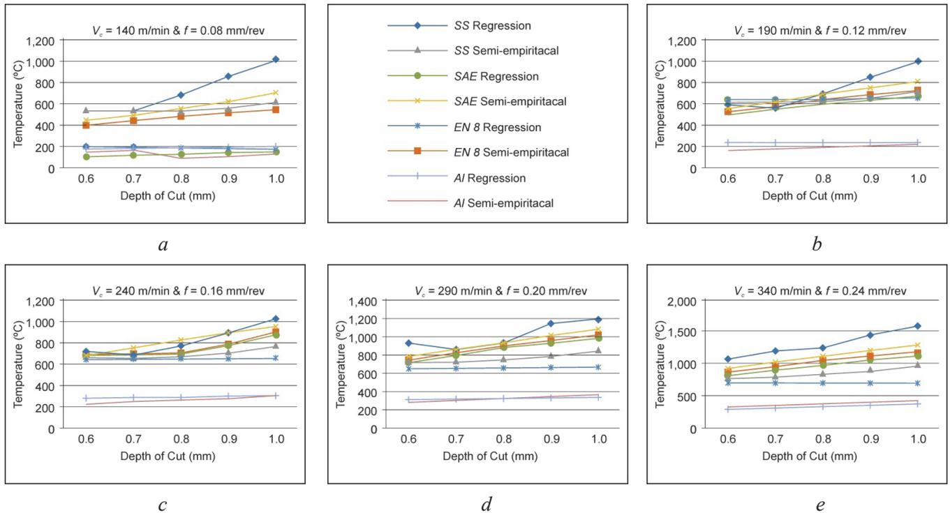
Fig. 9. Effect of depth of cut on cutting temperature at different feed rate and cutting speed for all material using  $TiAlN$ -coated tool
