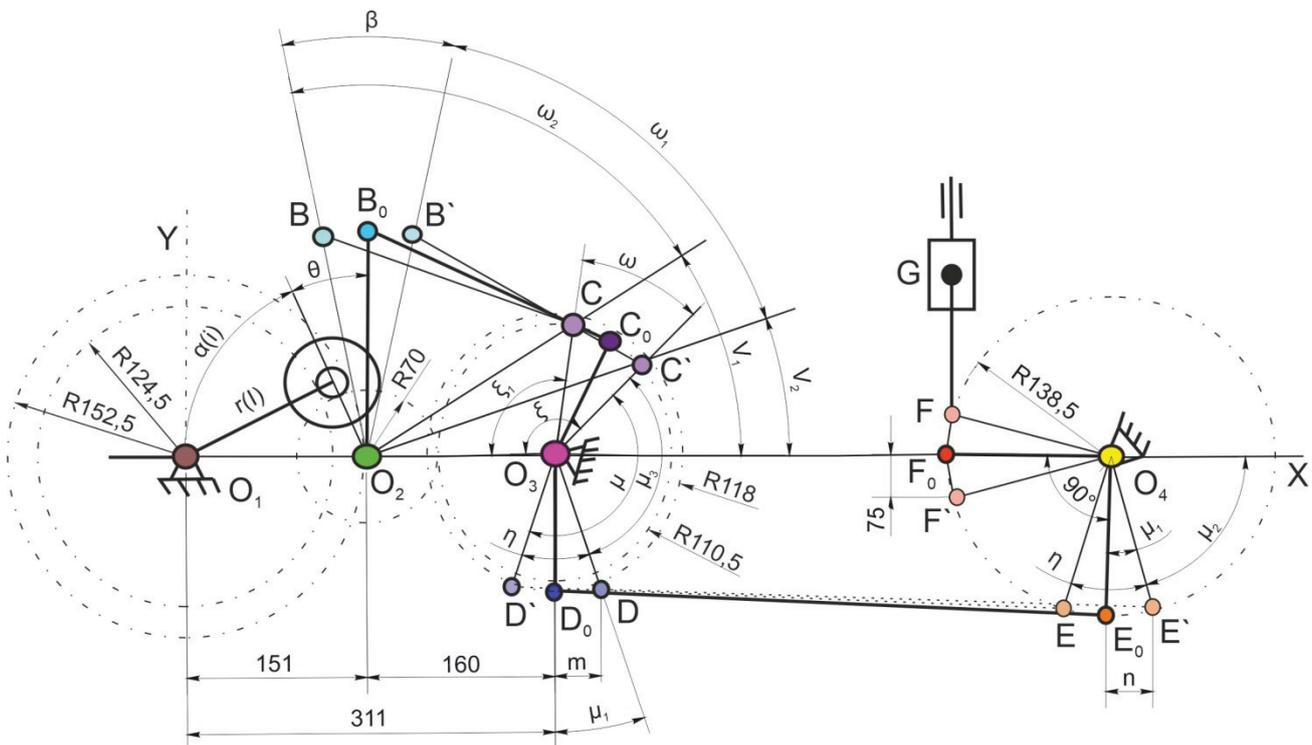
Fig. 2. Kinematic scheme of the heddle drive mechanism
