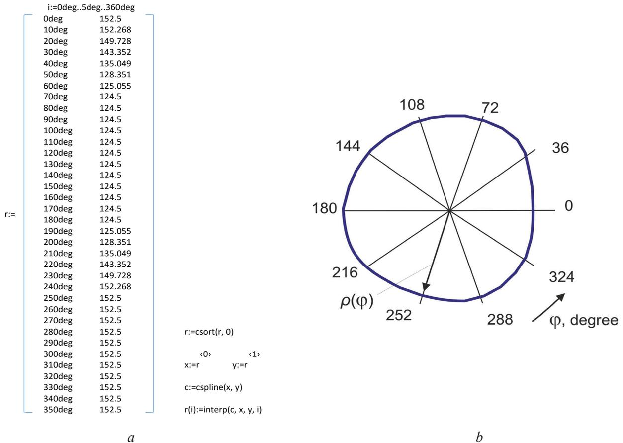
Fig. 6. The matrix of values of radius vectors and the shape of the cam profile:
