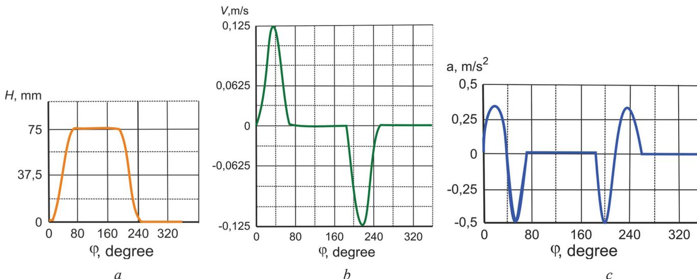
Fig. 14. Kinematic characteristics for point *F*:
