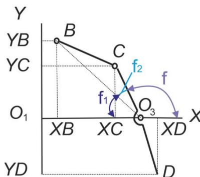
The coordinates of point  $B$  are found as projections on the  $X$  and  $Y$  axes:
