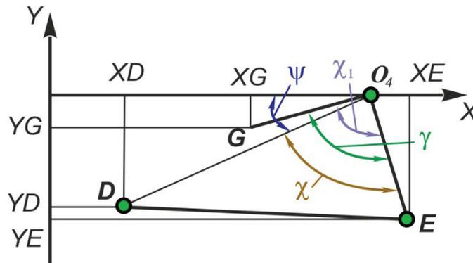
Fig. 9. The second-class first-type Assur group, which is part of the general scheme of the heddle motion mechanism
