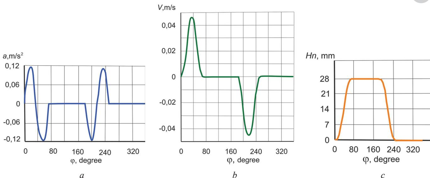
Fig. 4. Graphs of kinematic characteristics' analogs for the center of the roller:
