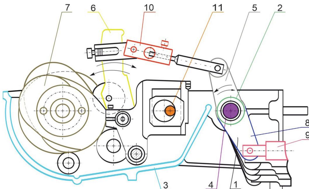
Fig. 1. The design scheme of the heddle motion consists of several components, including a two-arm lever (1), a hub (2), a body (3), a shaft (4), a top arm (5), a roller lever (6), eccentric drive (7), a bottom arm (8), a horizontal rod (9), a connecting rod (10), eccentric mechanism (11)
