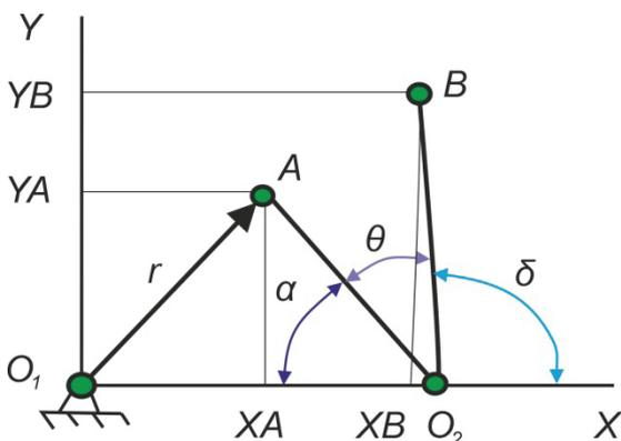
Fig. 7. The second-class first-type Assur group attached to the first-class first-type mechanism
