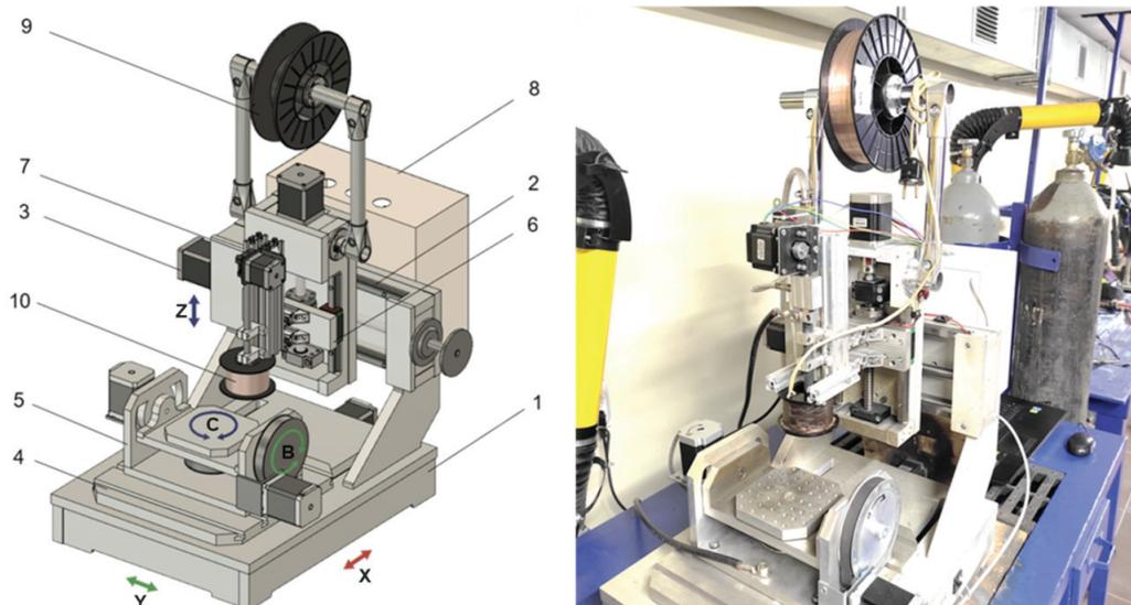
Fig. 1. Machine for wire-arc additive manufacturing on the basis of CNC machine:
