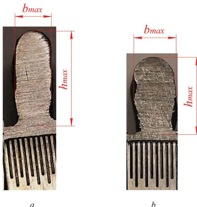
Fig. 5. Scheme for measuring the greatest width and height of the specimens surfaced:
