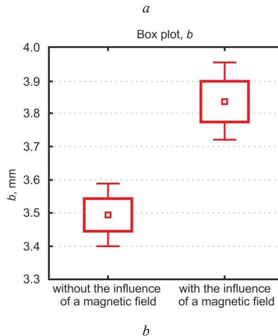
Fig. 10. Results of analysis of the influence of the longitudinal magnetic field on the walls width error of surfaced specimens:
