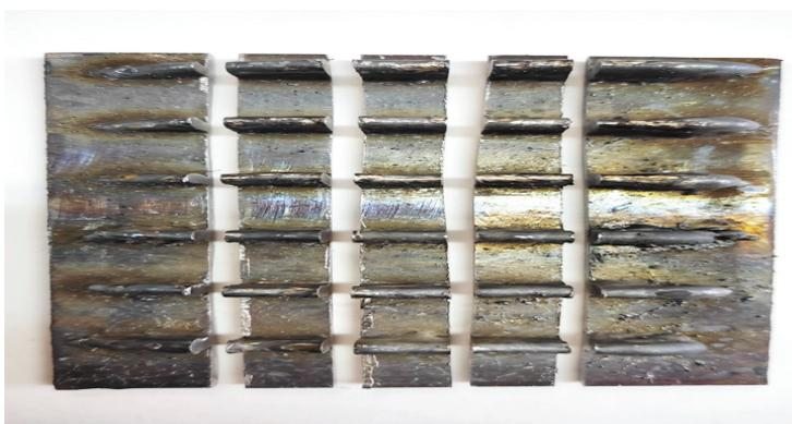
Fig. 4. Surfaced and cut specimens consisting of five layers
