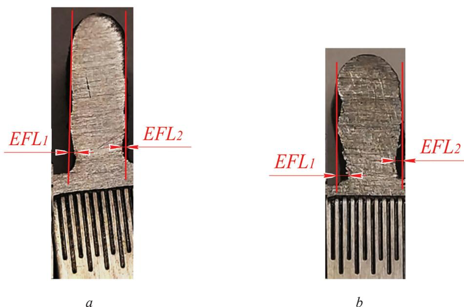
Fig. 7. Scheme for measuring the deviation from straightness of the specimens surfaced:
