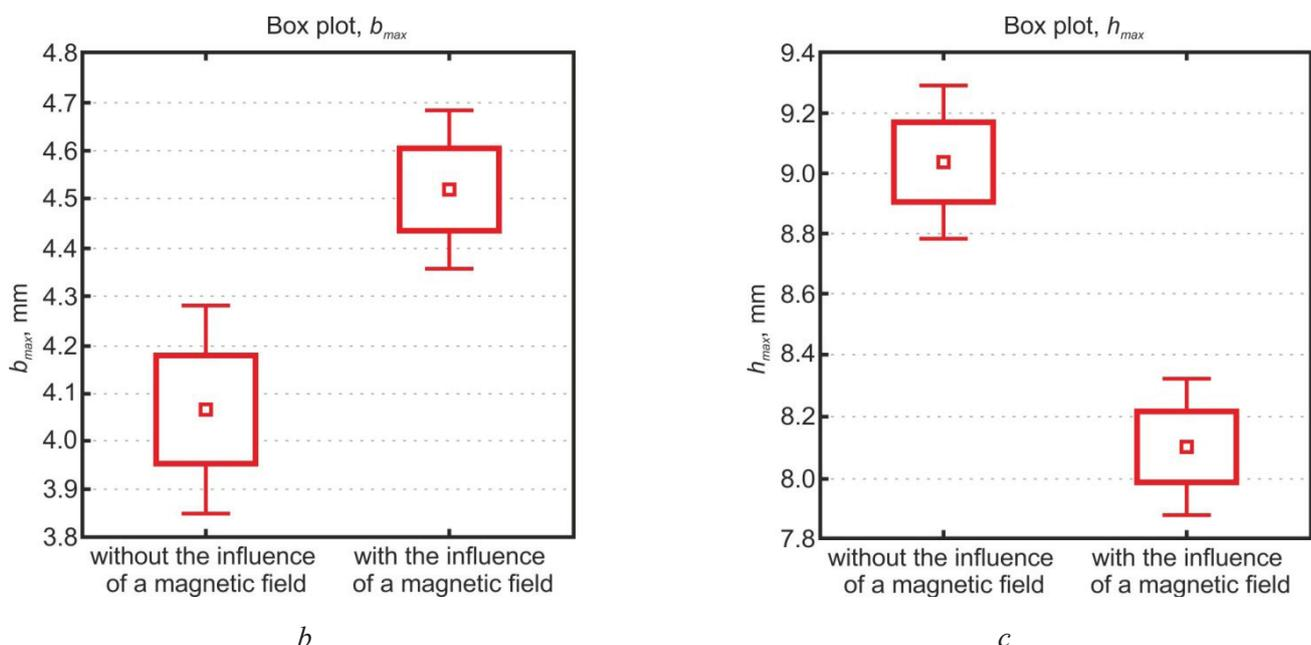
Fig. 6. Results of the analysis of the influence of the longitudinal magnetic field on the change of the overall dimensions of the surfaced specimens:
