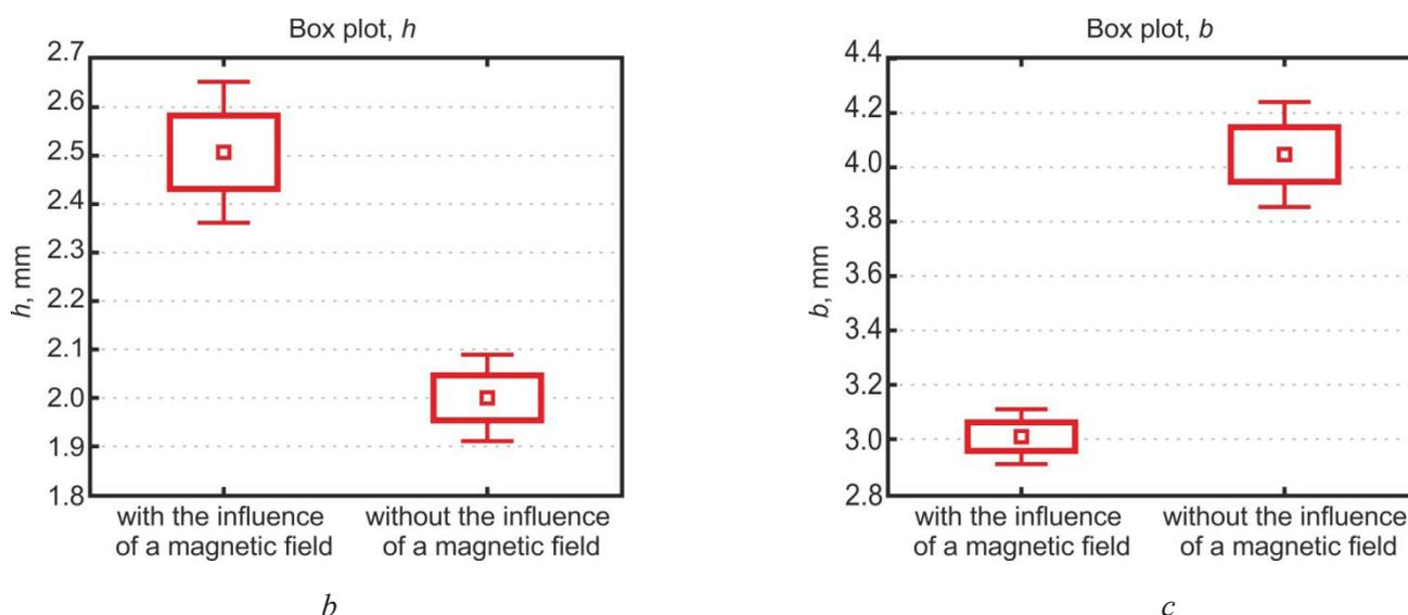
Fig. 3. Analysis of the effect of a longitudinal magnetic field on the change in dimensions of single surfaced layers:
