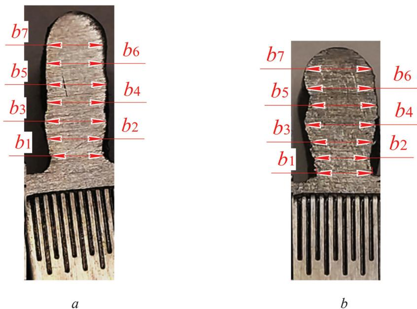
Fig. 9. Scheme for measuring the width of the surfaced specimens:
