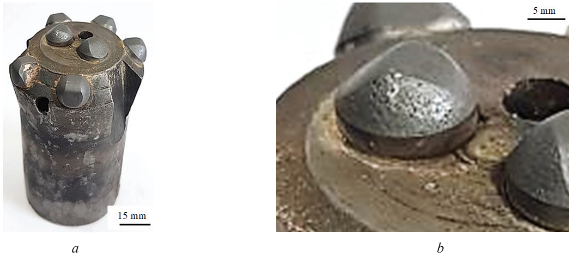
Fig. 1. Seven-cone drill bit type KNSh 40×25 manufactured by NPO , after operational tests during drilling of granite rock; drilling depth 18 cm (a); the condition of the surfaces of the teeth of the crown, characterized by porosity with depressions known as the formation of the “reptile skin” surface (b)
