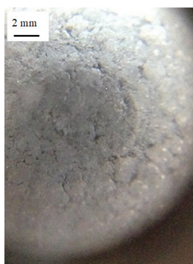
Fig. 12. Working surfaces of teeth of ballistic ( a ) and semi-ballistic ( b ) shapes
