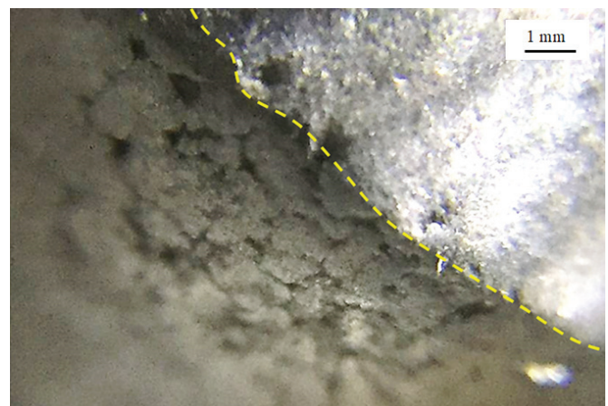
Fig. 2. Cross-section of the boundary of the surface of the tooth wear area with the tooth surface before wear: left – original surface; right – surface as a result of wear
