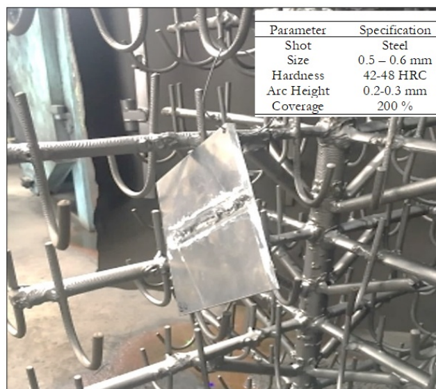
Fig. 4. Mounted specimen for shot peening
