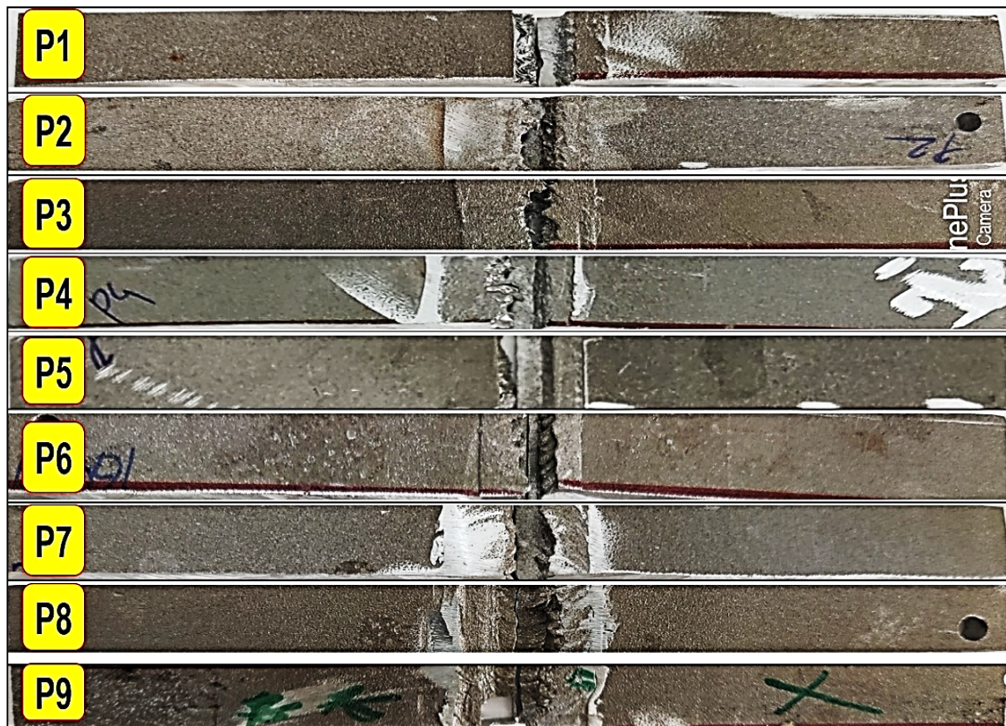
Fig. 8. Fracture behavior of the shot-peened UVaFSWed AA7075 joints
