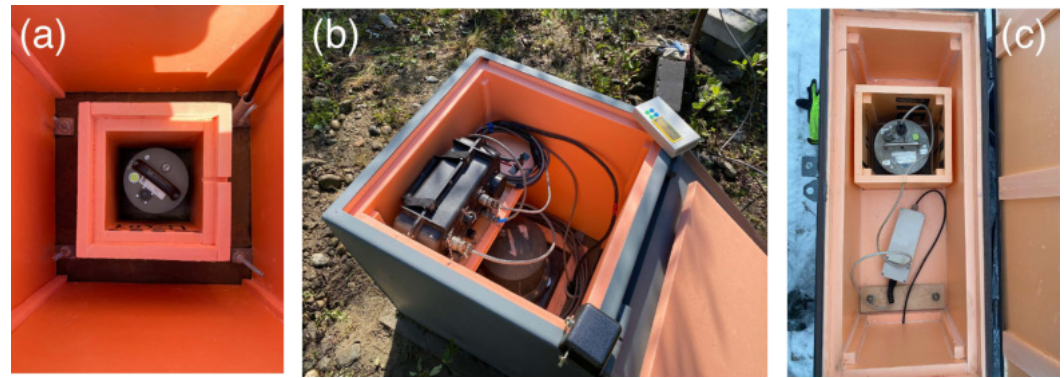
Figure 3. The seismic equipment within the insulated metal cases at stations Umba (a), Verkhnetulomsky (b), and Ogni Murmansk (c).
