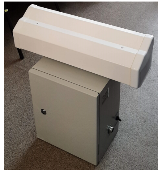
Figure 2: Photo of the X-band knife-like antenna beam ( 30^\circ \times 3.6^\circ ).
