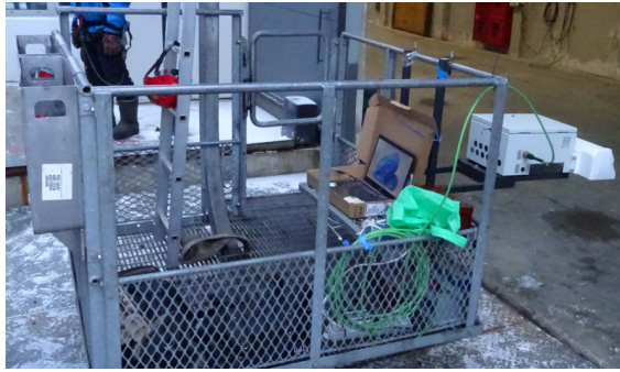
Figure 5: Technological trolley with installed radar before the experiment.
